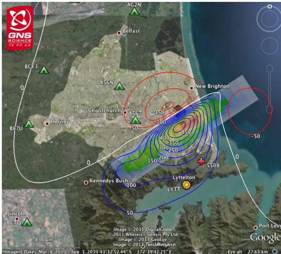
Figure 3-8. Preliminary model of the southeast-dipping fault (rectangular area) that ruptured across the southern part of Christchurch and northern Port Hills during the 22 February 2011 Christchurch earthquake. Colors on the fault plane indicate the amount of slip between the two sides of the fault. The contour lines indicate the amount (in mm) the land has risen (blue contours) or subsided (red contours) due to the slip on the fault. The white line is the contour where there was no change in height. The red, green and yellow colored symbols show some of the GPS stations whose displacements were used to derive the fault slip model (GNS Media Release, April 2011).
