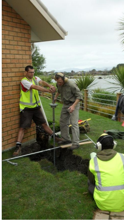
Figure 4-24. DCP test being performed adjacent to a house in Bexley after the M_w 7.1 , 4 September 2010 Darfield earthquake. Brady Cox is working the hammer. (13 Sept 2010, -43.51837^\circ , 172.72205^\circ )
