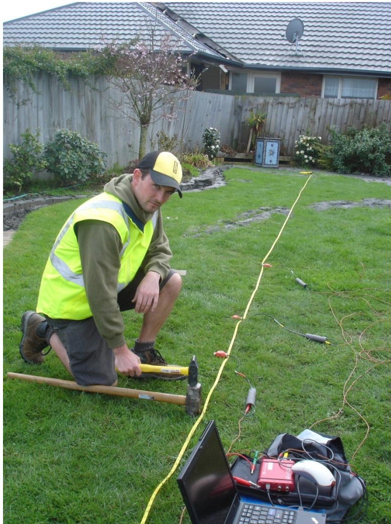
Figure 4-27. SASW setup at a site in South Kaiapoi. Liam Wotherspoon working the hammer. (12 Sept 2010; -43.39001^\circ ; 172.66264^\circ )
