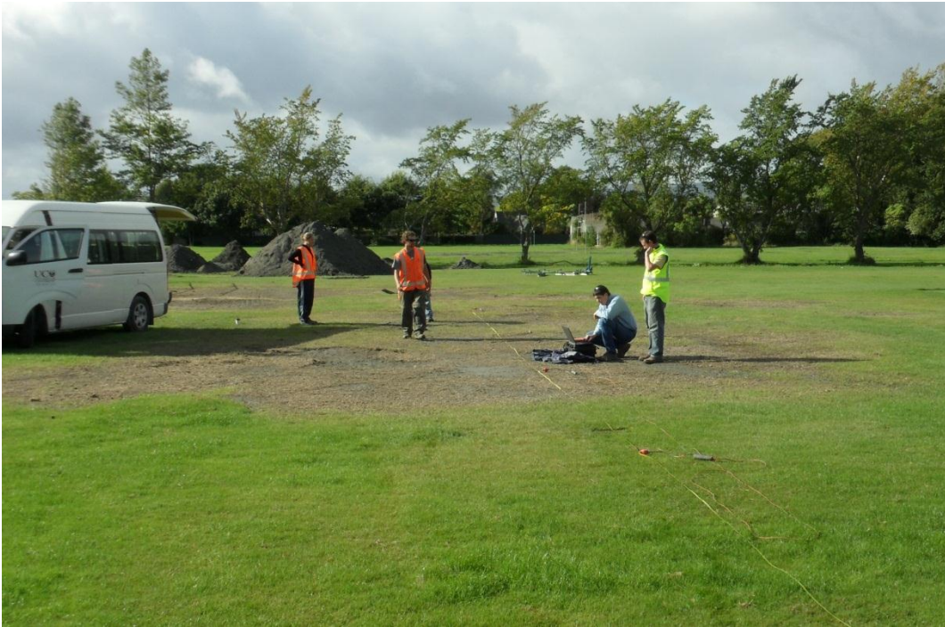
Figure 5-32. SASW array at St. Andrews School test site. (-43.50953°, 172.61291°)
