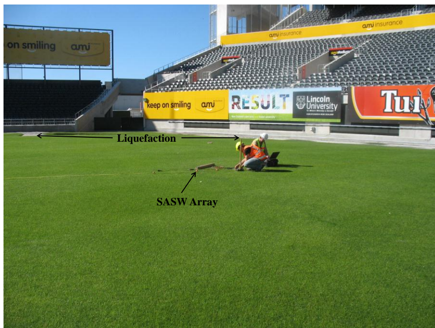
Figure 5-10. SASW array at AMI Field. ( -43.54161^{\circ} , 172.65452^{\circ} )
