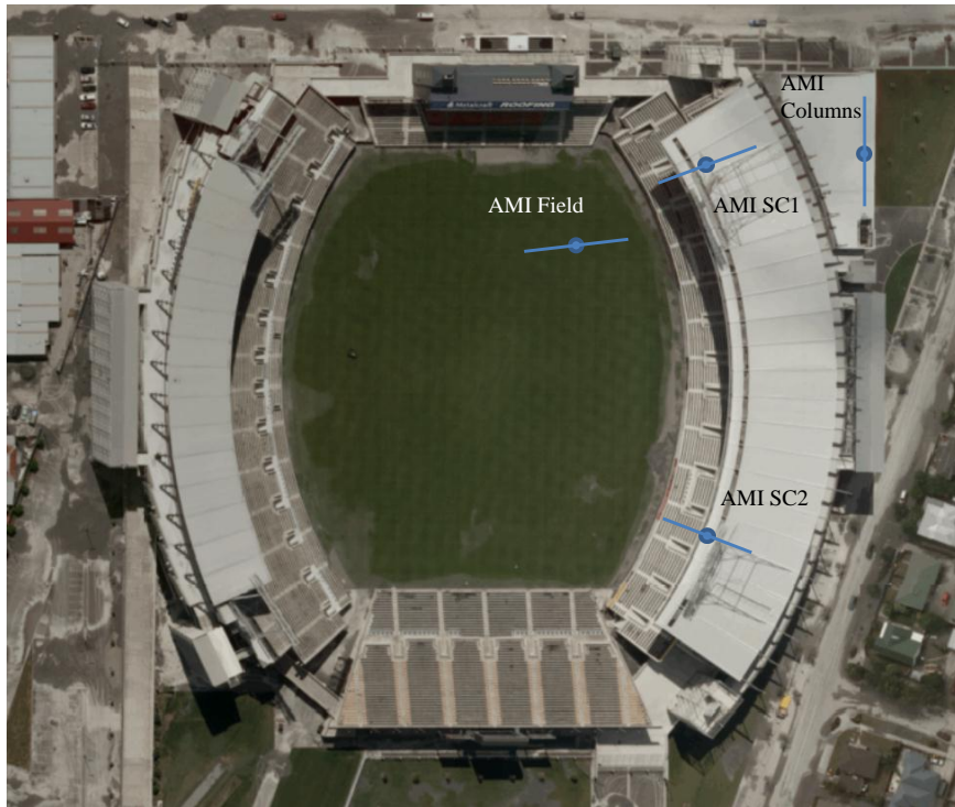
Figure 5-9. Aerial photo of AMI Stadium indicating the locations of four SASW arrays: AMI Field: -43.54161^{\circ} , 172.65452^{\circ} ; AMI Columns: -43.54128^{\circ} , 172.65562^{\circ} ; AMI SC1: -43.54138^{\circ} , 172.65501^{\circ} ; AMI SC2: -43.54236^{\circ} , 172.65514^{\circ} .
