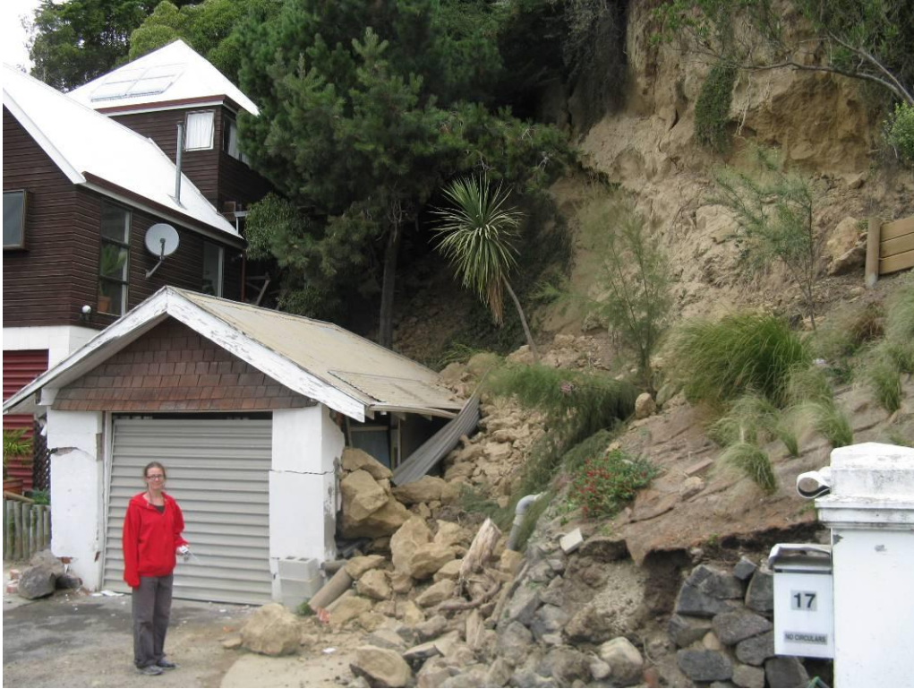
Figure 9-4. Blocks of loess that fell from a 10 m road cut on Mt Pleasant ( -43.5565^{\circ} , 172.7147^{\circ} ).
