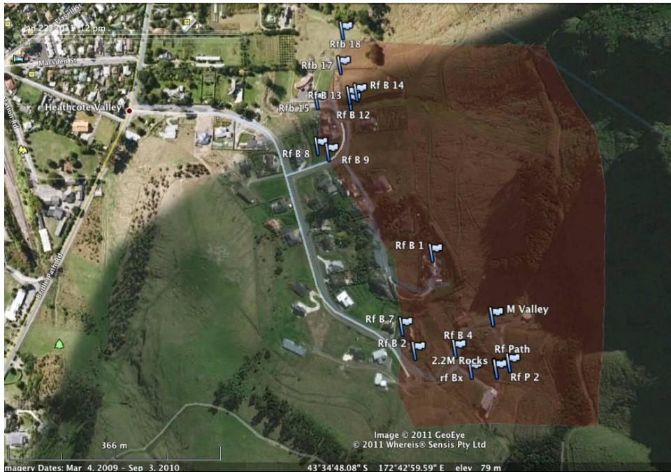
Figure 9-14. Boulder locations mapped 22-25 February 2011 in Morgan's Valley. Red shaded area was identified as the potential rockfall hazard zone.
