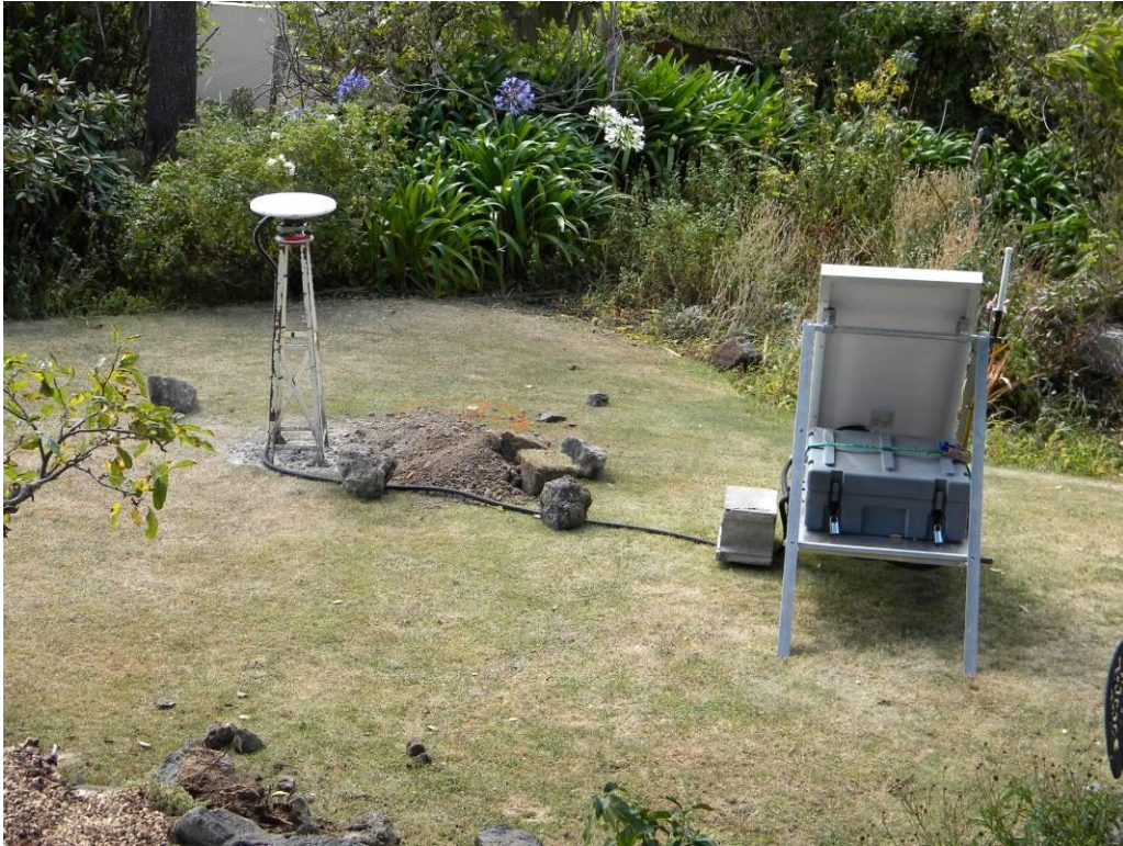
Figure 9-25. Continuous GPS monitoring station installed on Clifton Terrace by GNS to monitor post-earthquake slope movement ( -43.56586^\circ , 172.75272^\circ ).
