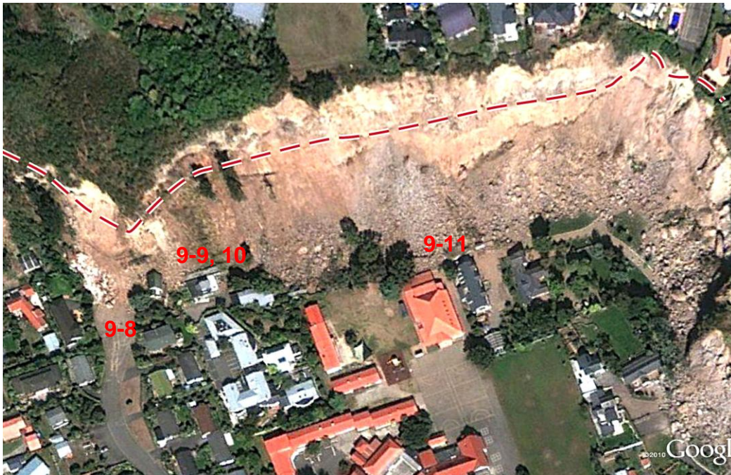
Figure 9-7. Pre-Earthquake (4 March 2009; top) and post-earthquake (23 February 2011; bottom) Google Earth GeoEye imagery oblique views of cliff walls in Redcliffs. Red line shows approximate pre-earthquake top of cliff. Location of photographs on Figures 9-8 to 9-11 shown on lower image.
