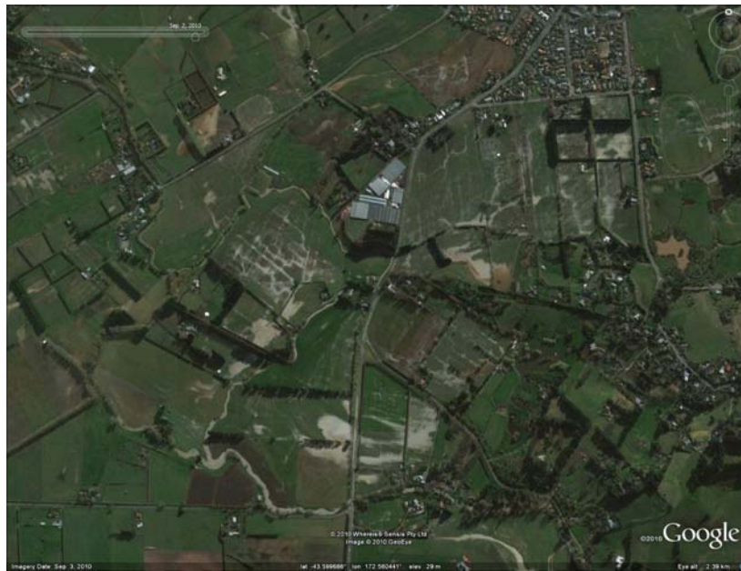
Figure 4.22 Part of Halswell as imaged by GeoEye after the earthquake. The ejected sand is accompanied by considerable volumes of water forming mini-lakes having a similar color to the ejected sand. From the left to the right edge of the image is ~2.74 km (Google Inc., 2010). (-43.598349°, 172.566383°)
