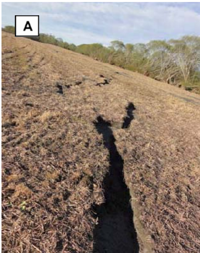
Figure 4.29 Massive lateral spreading at South Kaiapoi: (a) Sand boils and area affected by lateral spreading around Courtenay Lake (from a helicopter flyover on Friday, 10 September 2010); and (b) Large lateral spread cracks in farm land (at B: -43.3941389^\circ , 172.659750^\circ ).
