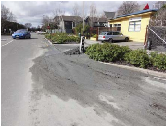
Figure 4.12 Evidence of limited/partial liquefaction in areas of Christchurch: (a) Evidence of liquefaction at Peterborough St - Madras St (CBD) ; (b) Sand boil in the foundation soils of a transmission tower (sub-station northeast of Greers Rd – Ruddenklau Ln, Bishopdale) (-43.4928055°, 172.5918055°).
