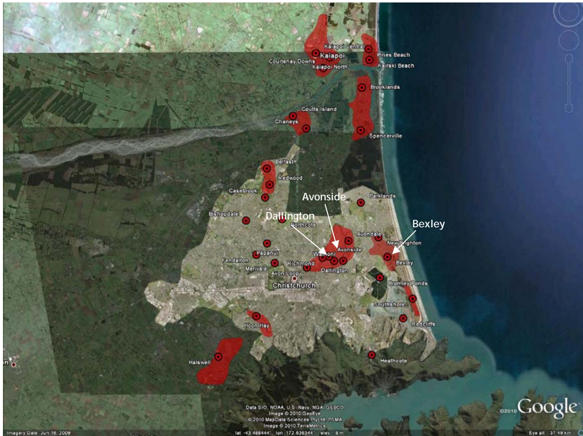
Figure 4.3 Areas of observed liquefaction (red shaded regions and red points) in Christchurch due to the 2010 Darfield earthquake (the liquefaction map is based on surface manifestation of liquefaction visible in aerial photographs and compiled evidence from ground surveys).
