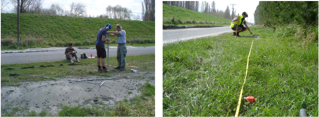
Figure 6.13 Photos 7 and 8: DCPT (left: -43.425137^\circ , 172.628619^\circ ) and SASW test (right: -43.424342^\circ , 172.630473^\circ ) performed in areas that did and did not liquefy along the levee on Coutts Island Rd. The locations of these photographs are denoted in Figure 6.4.
