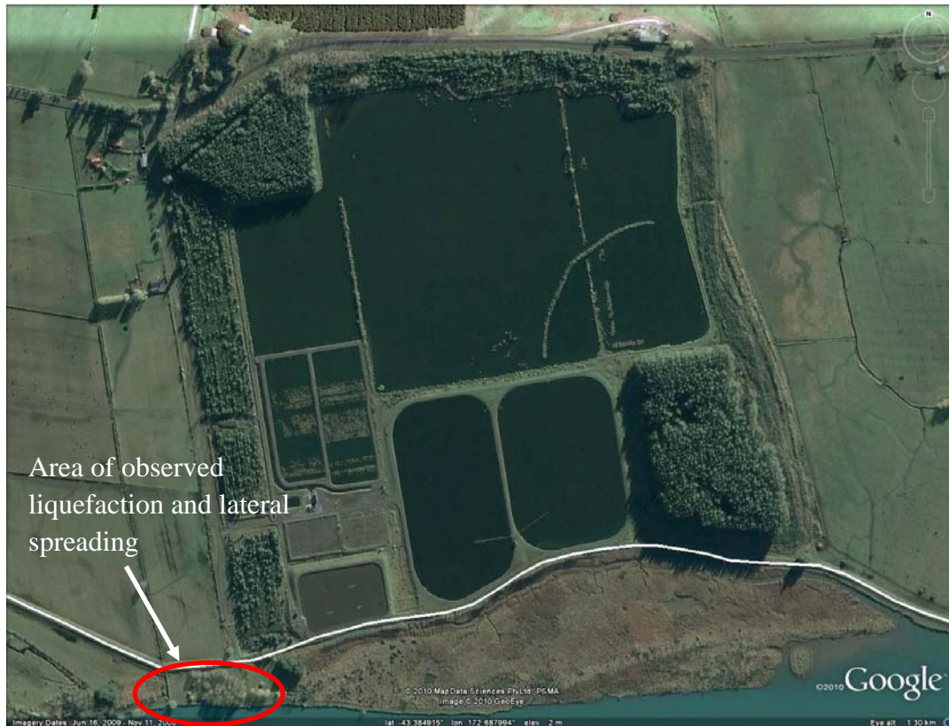
Figure 6.29 Aerial image of the Kaiapoi Sewage Treatment Plant. The southern perimeter (~0.6 km) of the oxidation ponds (bottom of image) forms the levees of the northside of the Waimakariri River. The distance from the left to the right edge of this image is ~1.5 km. (-43.384583°, 172.688240°)
