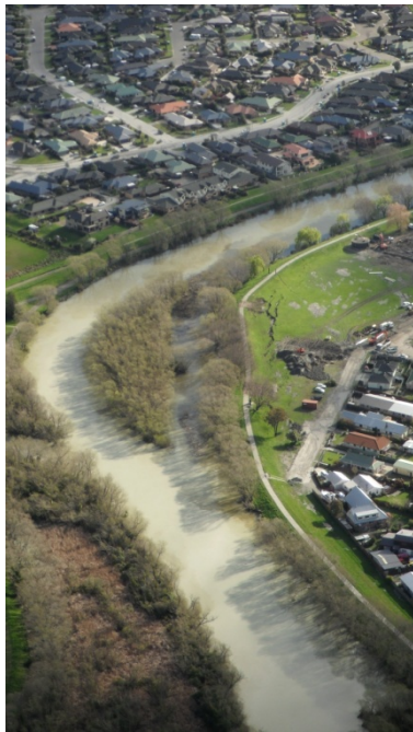
Figure 6.24 Photos 23 and 24: Aerial photographs of lateral spreading of levees on the north bank of the Kaiapoi River. The locations of these photographs are denoted in Figure 6.4. (left: -43.387389°, 172.666173°; right: -43.386875°, 172.672297°)
