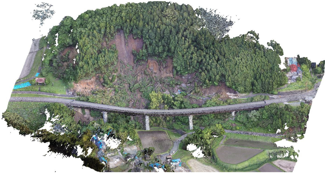
Figure 8-6. Screenshot of the Route 28 bridge and landslide 3D point cloud model developed from UAV-based video imagery (32.84236° N 130.92888° E).
