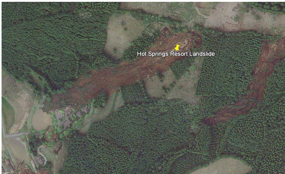
Figure 5-9. Google Earth image of the landslide, the hot spring resort was at the tail end of the landslide runout on the left, with the source area on the right.
