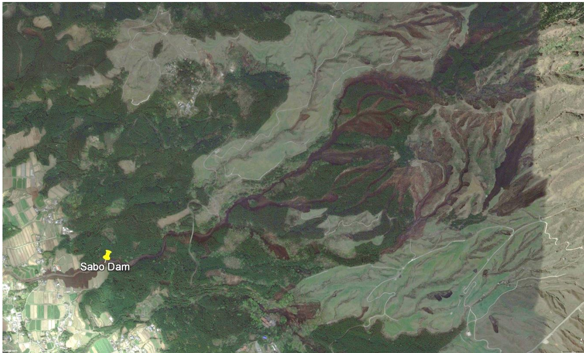
Figure 5-12. Google Earth image of the dam (located at the pin drop), the runout past the dam on the left, and the large ~2.5 km long, ~1 km wide source area to the right.
