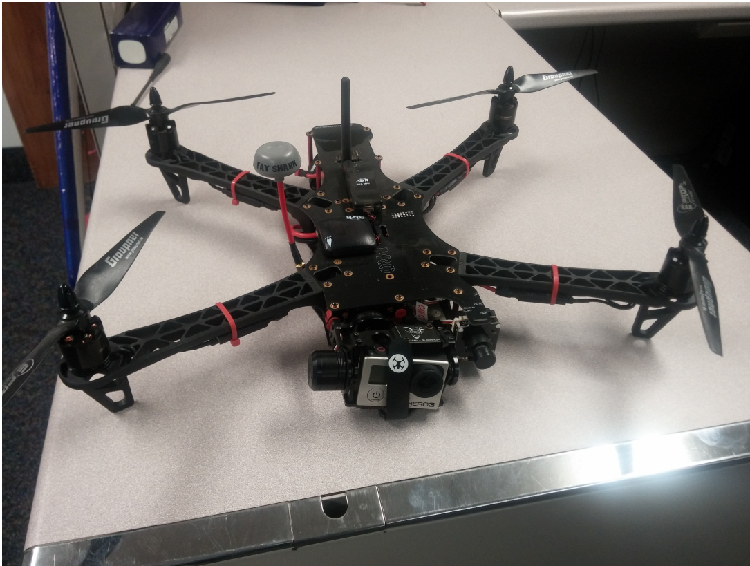
Figure 8-3. Discover Pro UAV manufactured by Team Blacksheep. The sensor shown is a GoPro Hero 4 Silver Edition.
