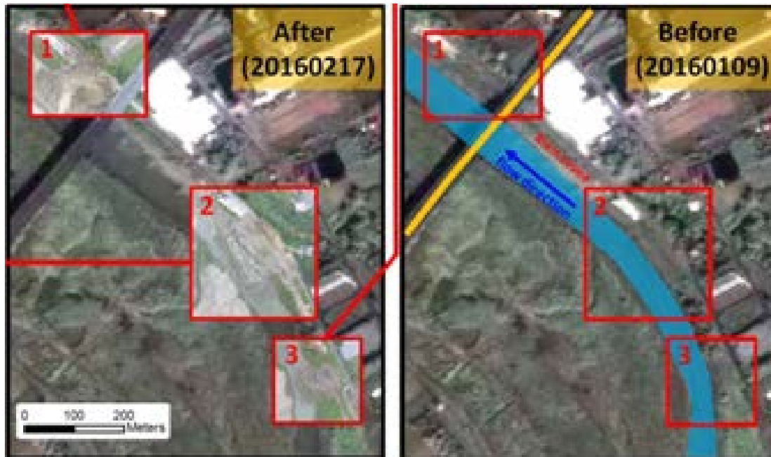
Figure 8-2: Pre- and Post-Failure Geometries of the Levee Slopes.
