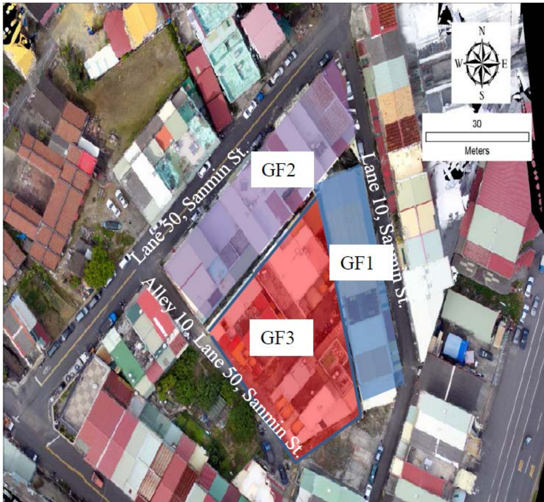
Figure 7-29: Ground failure index assessment of Xinshi site (By C.C. Tsai).
