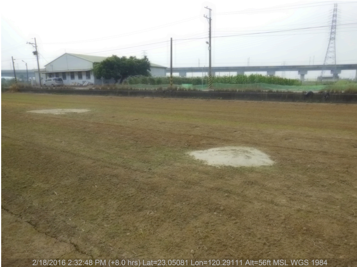
Figure 7-32: Open Field Liquefaction in Xinghus (THSR Viaduct in Background) ( 23.05081, 120.29111 ).
