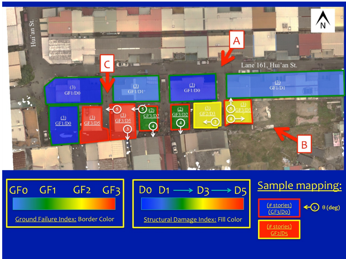
Figure 7-6: Assessment of ground failure – structural damage index (A, B, C denote images shown in Figures 7-7, 7-8, and 7-9, respectively). (center of region at: 23.0254°, 120.2074°).
