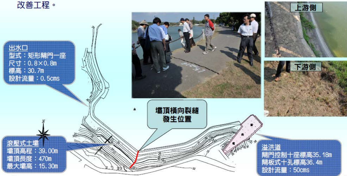
Figure 9-12: Earthquake Induced Transverse Crack from 2010 Jiasian Earthquake.
