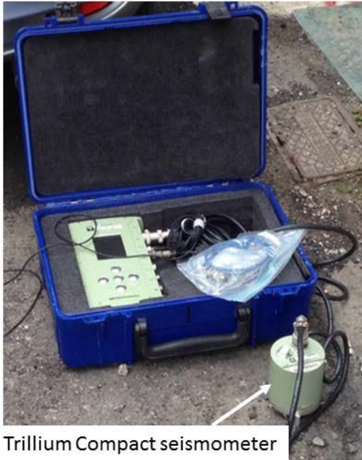
Figure 5-15: Photograph of a seismometer and data recorder provided by NHERI-EF@UTexas and a seismometer and data recorder provided by NCU.
