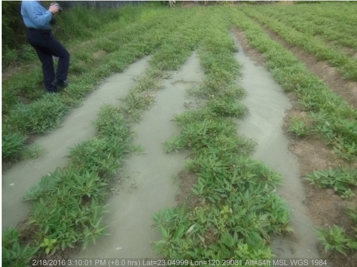
Figure 7-34: Sand Boil in Xinhua ( 23.04999 , 120.29081 ).
