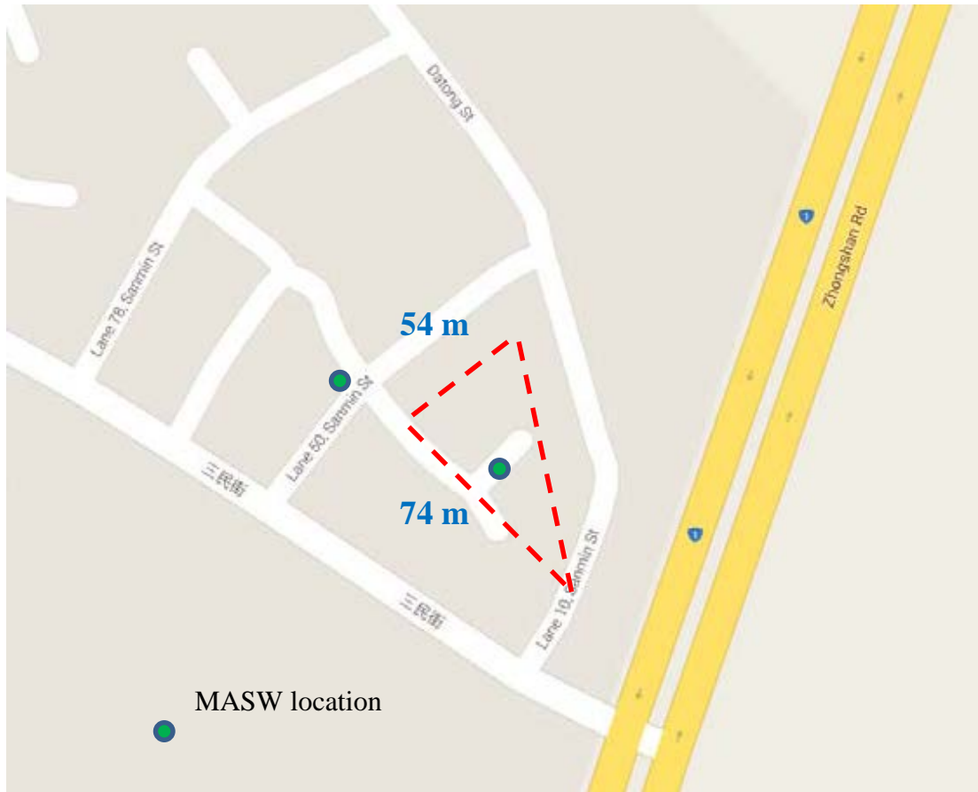
Figure 7-20: Approximate liquefied zone of the Xinshi site.
