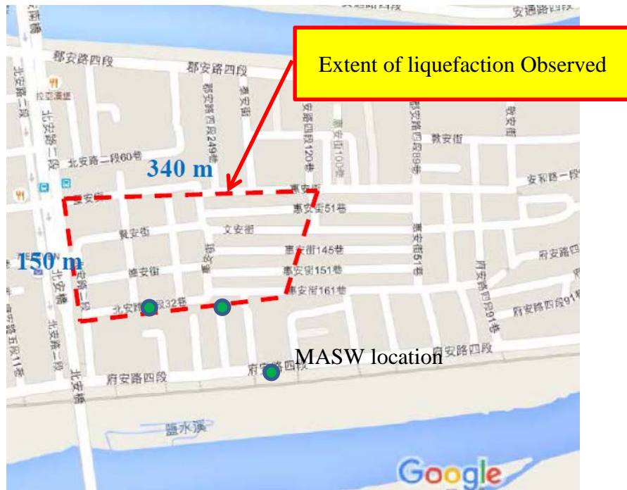
Figure 7-2: Liquefied zone of the Annan site ( 23.025585°, 120.207441° ).
