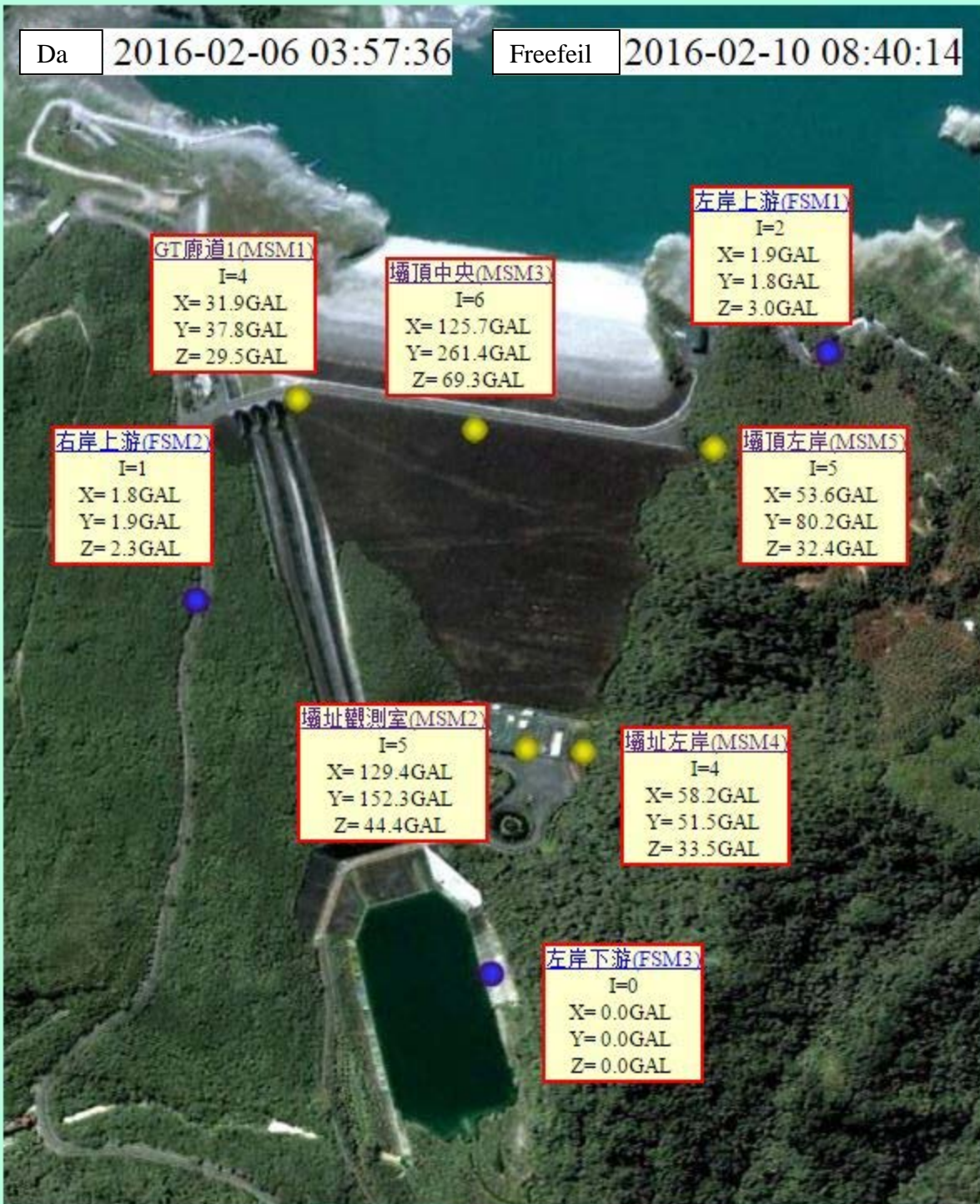
Figure 9-2: PGA Recorded on the Tseng Wen Dam Face (Freefield is from an aftershock).
