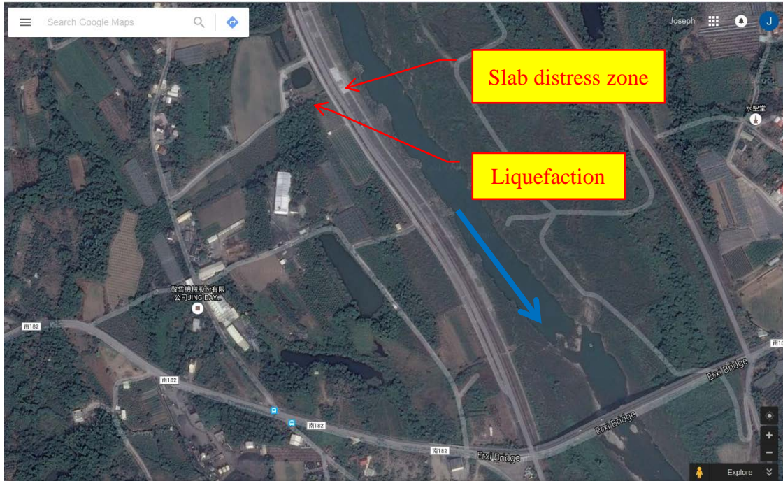
Figure 8-30: Aerial View of ErXi Bridge Levee Failure Site.
