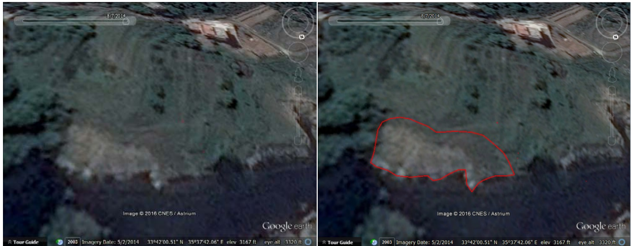
Figure 15: Change in color of grass as joints open and cut water supply prior to failing in August 2014- Red line presents 2015 failure zone (pictures form Google Earth Pro)
