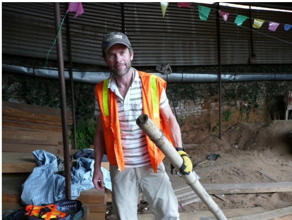
Figure 6-16. Bamboo sample of silty clay soil called “black cotton” in the Kathmandu Valley. ( 27.674816^{\circ} 85.362646^{\circ} ).
