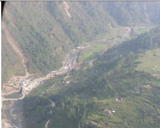
Figure 5-108 Dam site of a hydropower station near Barpak is vulnerable to potential landslide in the next rainy season or earthquake event.
