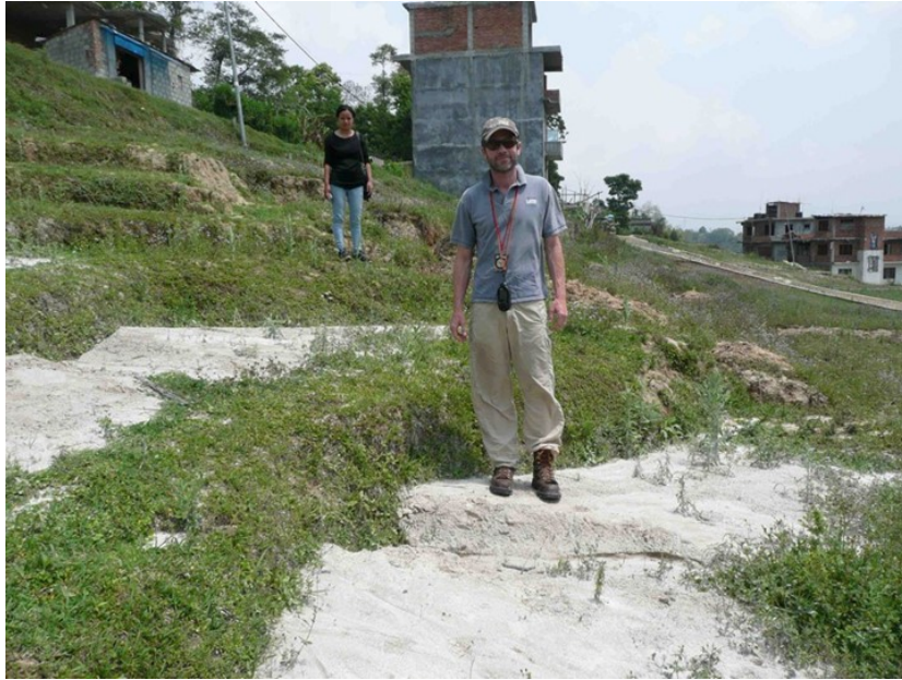
Figure 6-5. Liquefaction ejecta on steep terraced slopes (27.711025° N 085.262290° E). No lateral movement was observed. No damage to the building in the background.
