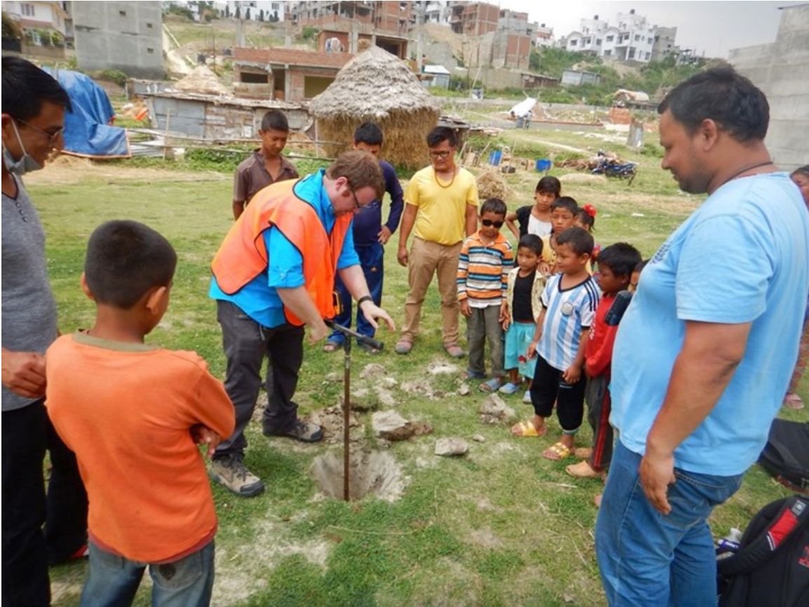
Figure 6-27. Hand augering a sand boil in Hattiban, 85.33441 N, 27.65567 E.
