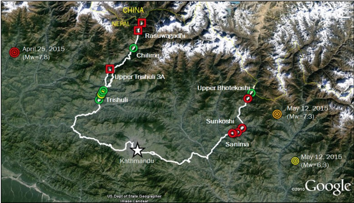
Figure 7-1 Hydroelectric plants visited by the GEER Team B. Squares indicate projects under construction. Circles mark completed projects. Red marks projects that sustained damage during the earthquake or were not operational due to earthquake damage, ongoing construction, or other issues. White marks the surface tracks of the GEER Hydro Assessment Team. The western track follows the Trishuli River and the eastern track follows the Sunkoshi River.
