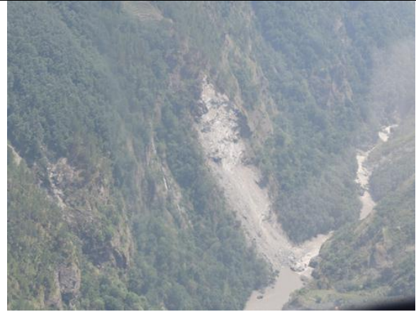
Figure 5-68 A large scale seismically induced landslide that partially blocked the Trishuli River.
