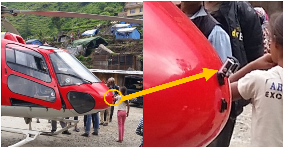
Figure 1-6 GoPro Hero Camera mounted on the nose of the reconnaissance helicopter, 27^{\circ}57'31.7''\text{N} , 85^{\circ}57'17.7''\text{E} .
