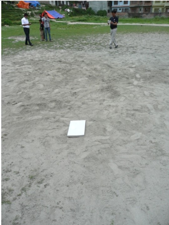
Figure 6-10. Large sand boil in a field at Manamaiju. The ejecta was a micaceous silty fine sand. (27.745523° N, 85.302223° E).
