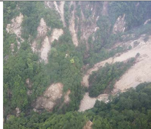
Figure 5-109 Seismically induced landslides near Barpak blocked the natural flow of a stream.
