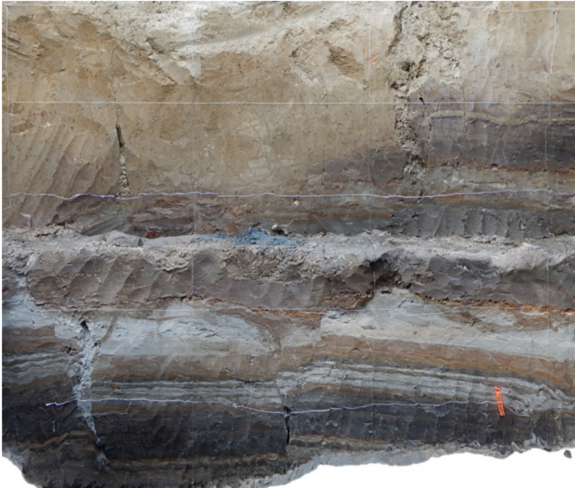
Figure 6-21. Cross section perpendicular to scarp at EMT09. Horizontal and vertical spacing of the string is 0.5 m and 1.0 m, respectively (27.675524 N, 85.363083 E).
