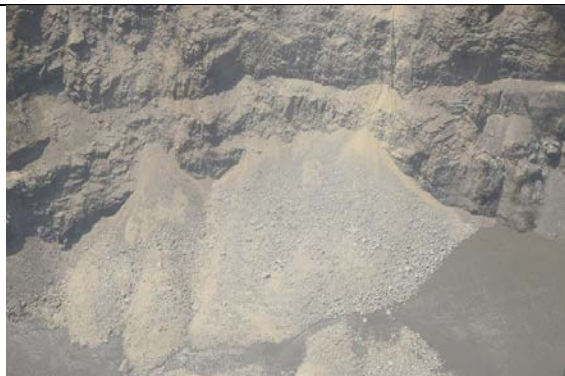
Figure 5-71 Closer view of the landslide dam at the Trishuli River (28°14.9'0"N 85°27.6'0"E)
