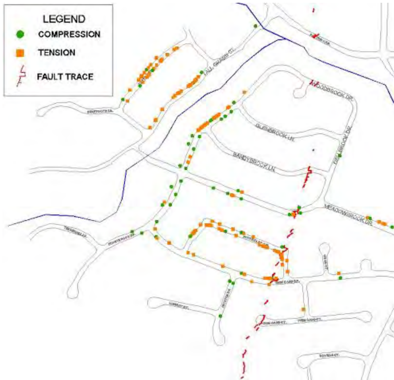
Figure D-2: Observed and measured tension (orange) and compression (green) locations; produced in AutoCAD; [NSF-GEER; Luque, R.; Wagner, N.; processed 9/5/14]
