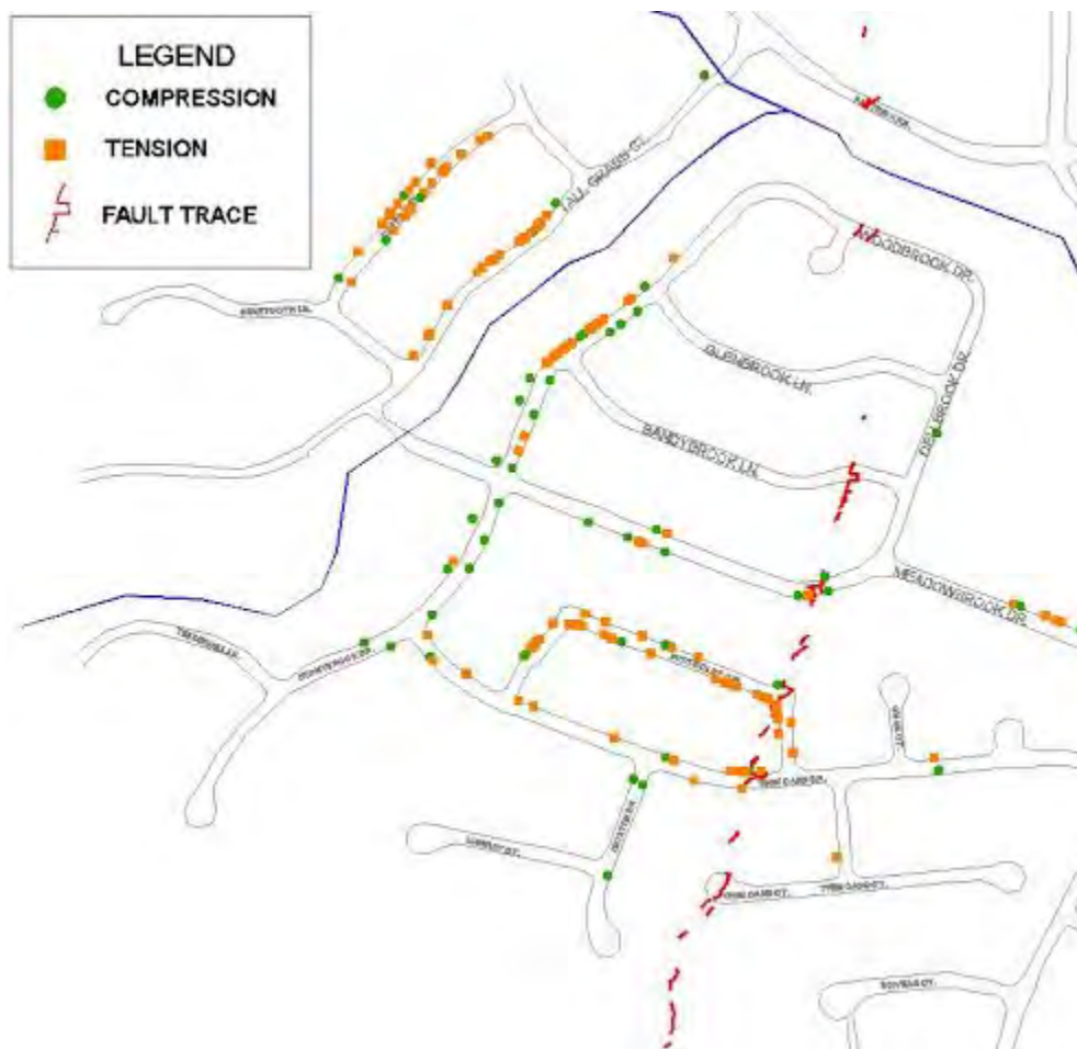
Figure 5.6: Observed and measured tension (orange) and compression (green) locations; produced in AutoCAD; [NSF-GEER; Luque, R.; Wagner, N.; processed 9/5/14]
