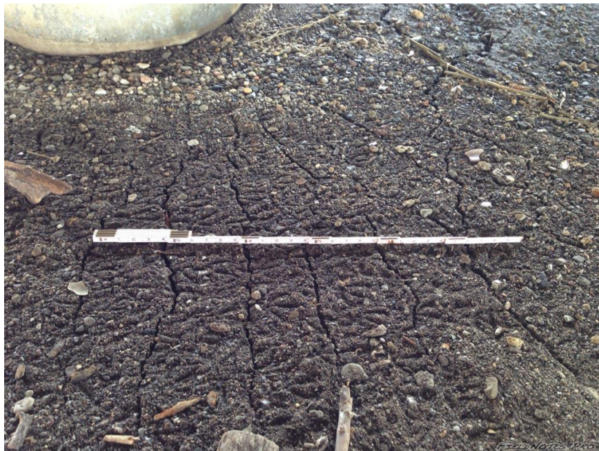
Figure 6.8: Ground cracking due to liquefaction in Napa River point bar below 3 rd St. Bridge, between the two columns of the eastern pier. [NSF-GEER; N 38.2980 W -122.2840; 08/24/14 14:44]
