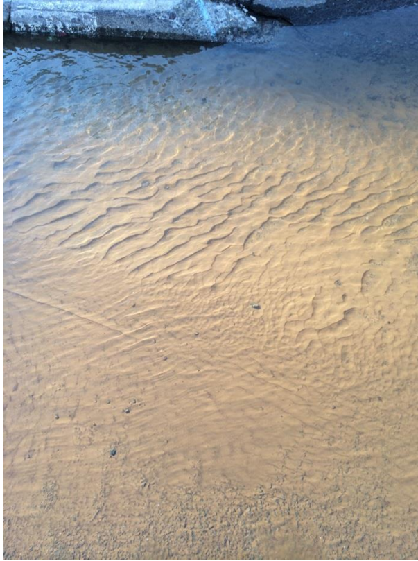
Figure 6.13: Soil ejected from water main break in Arroyo Dr. [NSF-GEER; N 38.3008 W -122.2894; 08/24/14 16:34]
