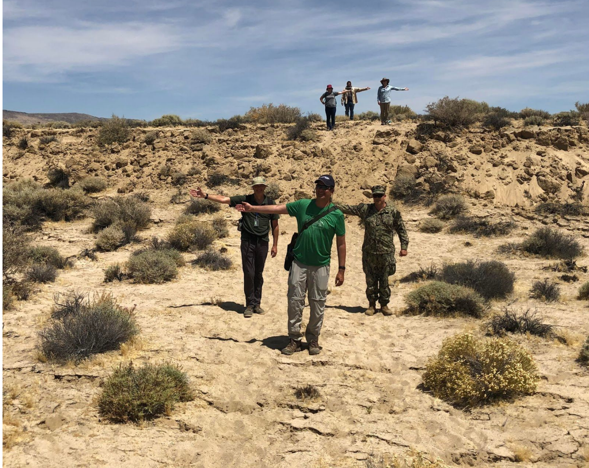
Figure 5. All six people are standing on a surface that was nearly flat prior to the M7.1 earthquake, and here the fault rupture offset the ground surface vertically by one to two meters, forming a fault scarp. The lateral offset of about 3 to 4 m shifted a dirt road set of tracks to the right (see Fig. 9 for additional details at this site). On each of the sides of the fault, three people are marking the same three features that have been offset; the center line of the road and each of the tire tracks. All are pointing to indicate the tectonic sense of right-lateral fault motion. (Credit; Photo by John Foster, US Navy; public domain).
