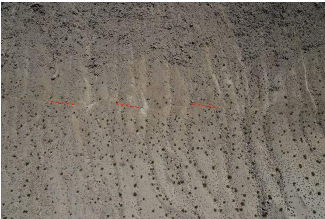
Figure 10. A series of nearly parallel and sharply incised small drainage gullies occur along a NW-SE oriented ridge line that lies from 1 km to 3 km southeast of the offset access road shown in Fig. 8. The roughly twenty such gullies shown in this photo are referred to as the “offset gullies”. The short dashed red line segments indicate the location of the mainshock fault surface rupture, which forms a bench as the fault cuts across this hillside, nearly perpendicular to these gullies. With high-resolution topography from the air photos already collected, and potentially from the airborne lidar in the future, geologists expect to be able to precisely measure fault slip variation along this section of the fault. Slip is known to diminish from approx. 1.8 m at the abandoned railroad tracks down to less than one meter at the SE end of the ridge where these gullies were found. So, it is expected that these gullies will afford a way to quantify the reduction in slip from NW to SE along this 2 km long section of the fault.
