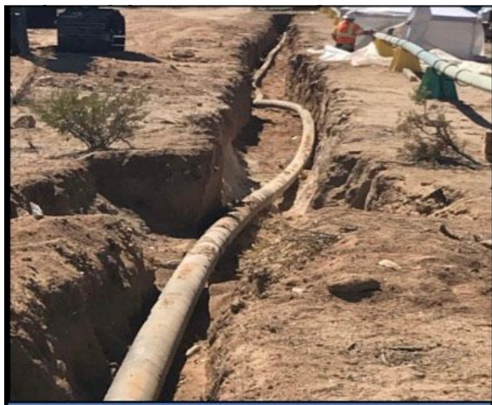
Figure 31. Deformed section of 10.75 inch steel gas pipeline following excavation at crossing of M7.1 fault rupture. The surface rupture width in this area was approximately 0.5 m. Photo from PG&E.
