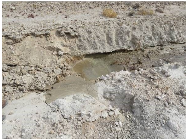
Figure 29. Pipeline damage at M6.4 surface rupture crossing. (a) broken pipeline at west side of rupture zone photographed before repair on 7/4/2019 (B. Brooks, USGS). (b) repaired pipeline at west side of fault zone. (c) repaired pipeline at east side of fault zone. (d) leak within fault zone after M7.1 earthquake. (35.6443, -117.5369)
