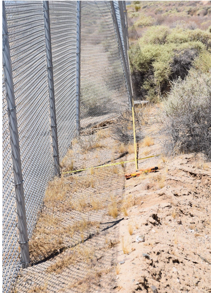
Figure 11. Offset fence line at southern Salt Wells Valley, just north of highway 178. The fence offset is 70 \pm 5 cm right-lateral sense. (photo by Jason R. Patton, CGS; Lat./Long. 35.6495, -117.4828)
